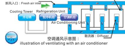
The main purpose of an air conditioner is either to cool or heat an occupied room and that's why to ventilate with an air conditioner cannot meet the minimum ventilation requirement.
